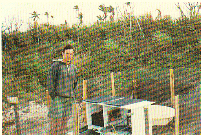
Figure 2. A typical field installation, this one located in Ha'apai, Tonga. The sensor is deployed in the fiberglass cylinder at the rear, and the batteries and recording gear in the plywood box, with solar panels mounted on top. Washington University graduate student Erich Roth inspects the site, which is complete with a "Tapu" sign and a fence to keep out marauding pigs and chickens.
